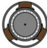
AC Induction Machine (ACIM)
